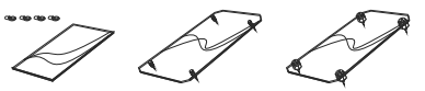
Additional Shelf (full size) (hwd 6 x 550 x 330) Isolation Platform (full size) (hwd 40 x 720 x 420) Floor Isolation Slab (full size) (hwd 90 x 720 x 420)
