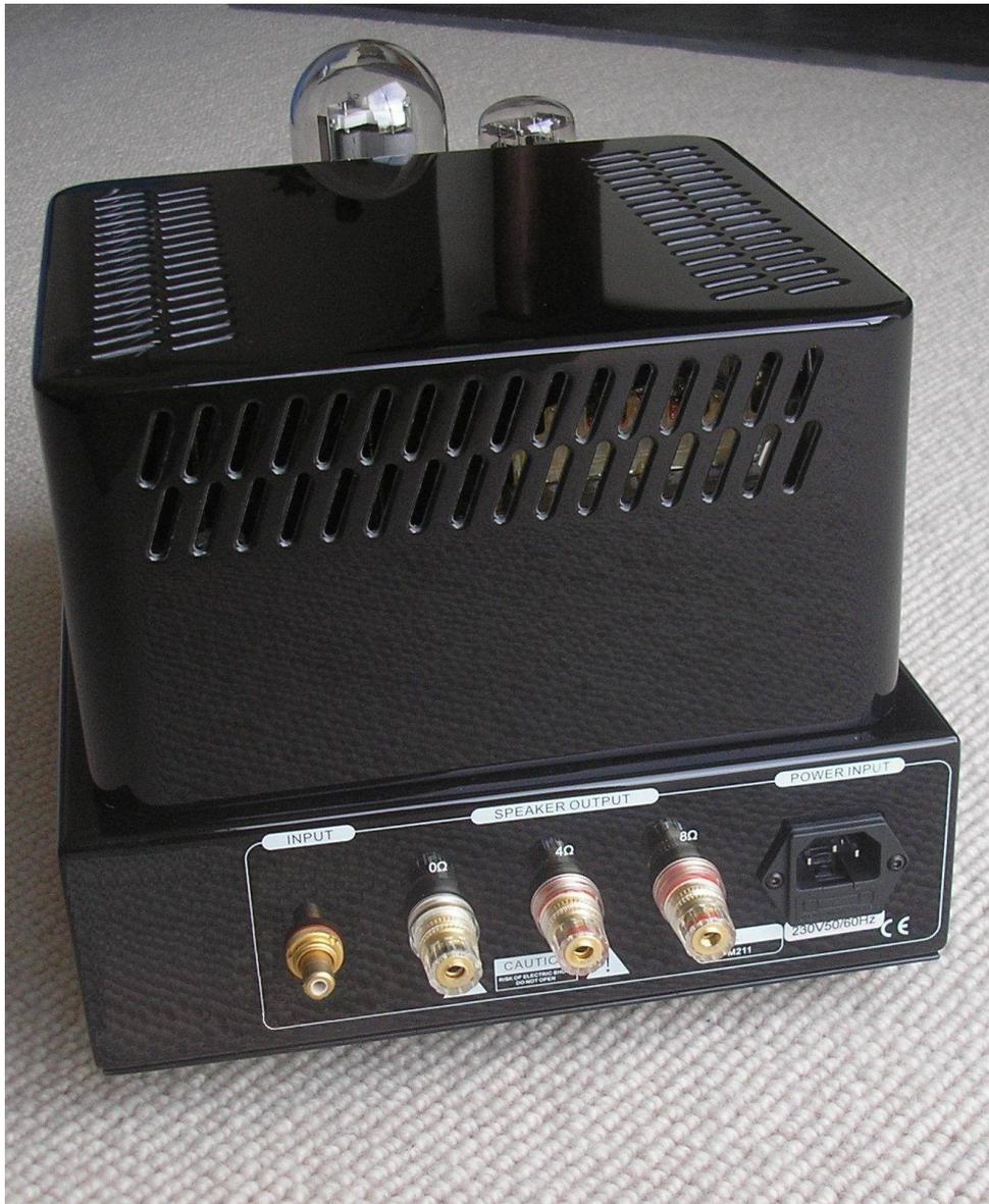
The other difficulty in using the 845 is in the design of a stage capable of cleanly delivering the voltage swing necessary at its grid to take it to full output. The M845 incorporates a driver stage based on the 6SN7 triode coupled via a custom wound, wideband, interstage transformer. The amplifier's input stage is directly coupled to this driver meaning that there are no coupling capacitors used in the circuit at all.
