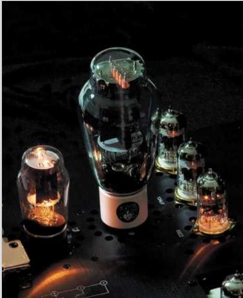
300B triode valve is part of the extremely sophisticated regulated power supply.
