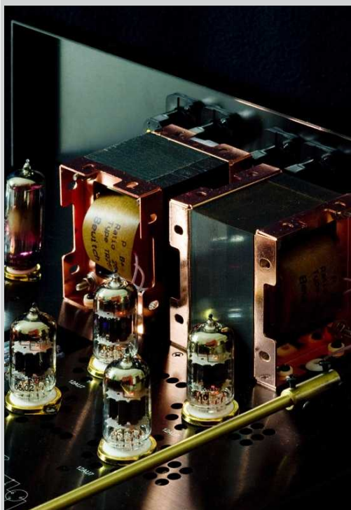
Output transformers allows the option of a true balanced output configuration.
