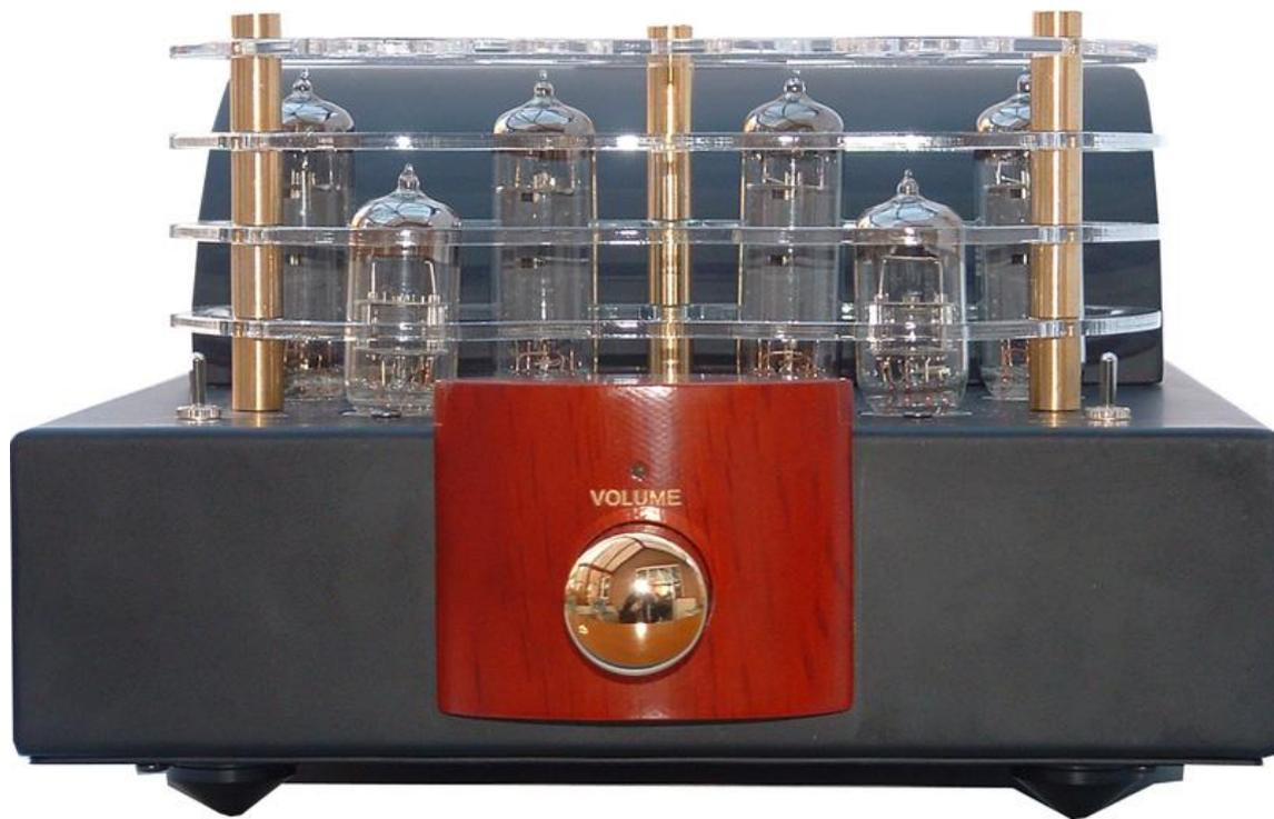
The amplifier uses the 6P14 output valves (an equivalent of the EL84/6BQ5) in an Ultra Linear push pull configuration. This arrangement gives a combination of power and clarity that is difficult to beat. There is a charming quality about the way this family of pentodes reproduce music. The amplifier uses an Auto Bias system, which means that replacement output valves should be fitted as matched pairs. There will be no need to reset or monitor bias conditions.
