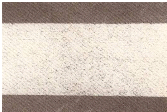
Crystal structure of conventional OF copper (x290).
